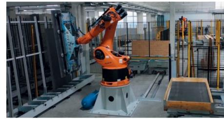
Vertical sheet loading increases warehouse capacity and reduces the risk of breakage.
